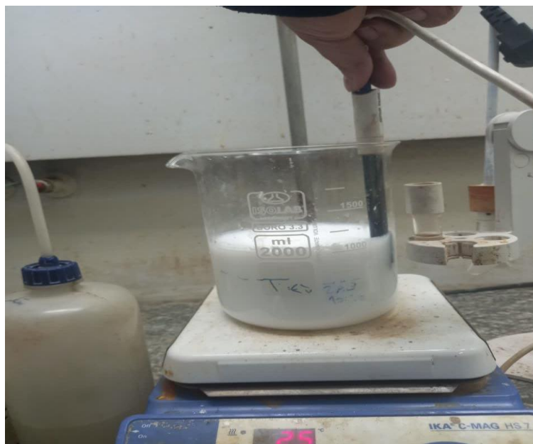
Figure 9 - Precipitation solution of magnesium hydroxide
