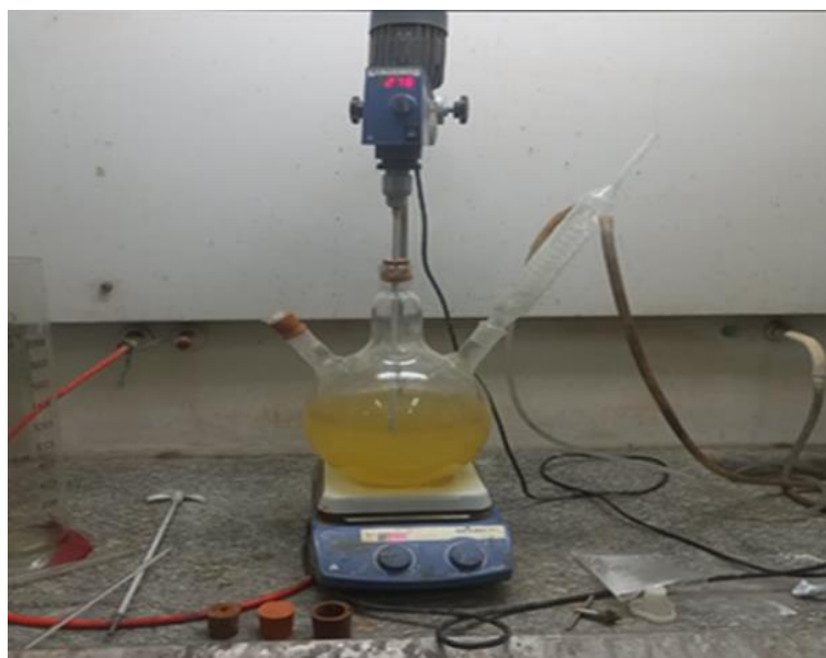
Figure 6 - Hydrochloric Acid Leaching of Calcined Dolomite
