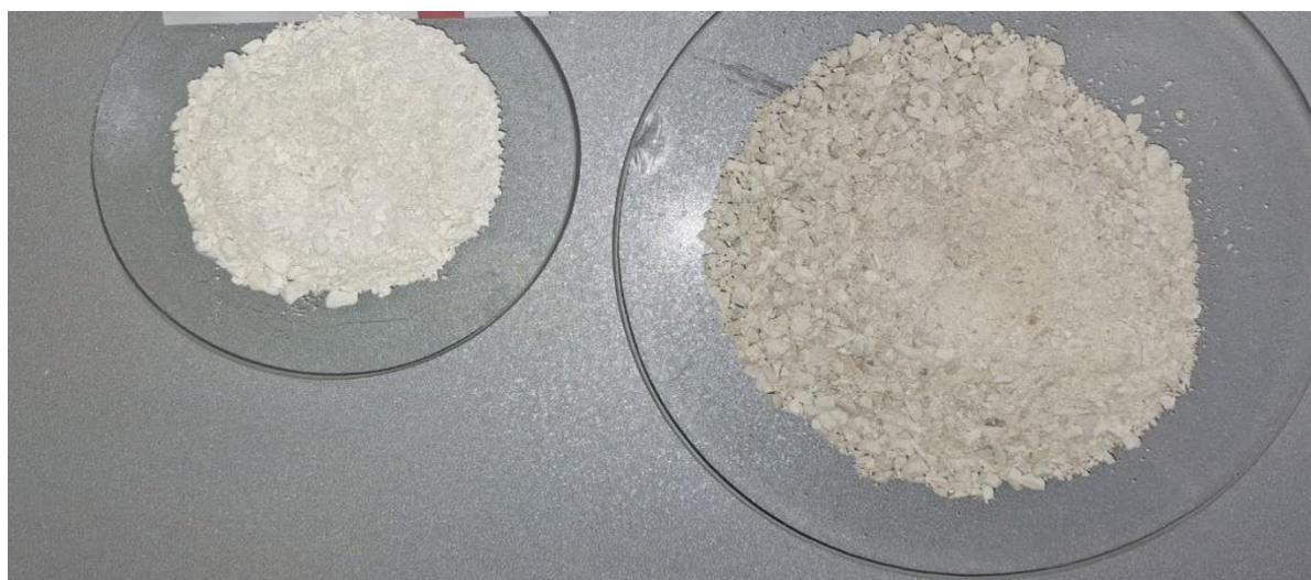
Figure 5 - Comparative images of the composite sample (right) pre-calcination state and (left) post-calcination state at 800°C.
