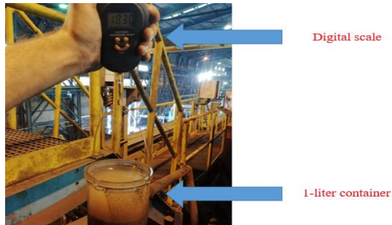
Figure 2 - Manual measurement of pulp solids percentage in situ.
