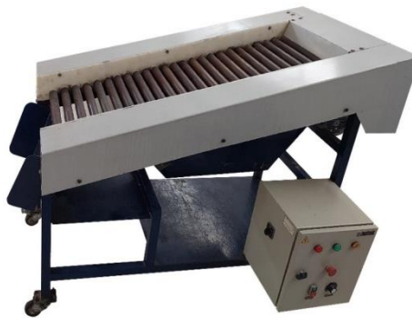
Fig. 4. Performing laboratory roller screen tests for classifying green iron ore pellets.
