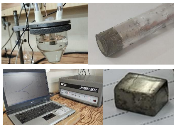
Fig. 2. Preparation steps of pyrite (WE) working electrode
