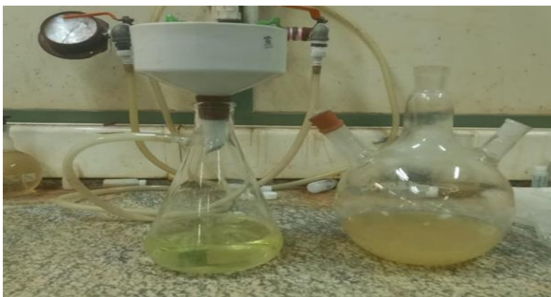
Figure 7 - Filtration of the Hydrochloric Acid Leaching Solution
